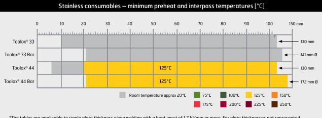
\*The tables are applicable to single plate thickness when welding with a heat input of 1,7 kJ/mm or more. For plate thicknesses not represented in the diagrams, contact SSAB for further information. If nothing else mentioned unalloyed and low-alloyed consumables apply.
